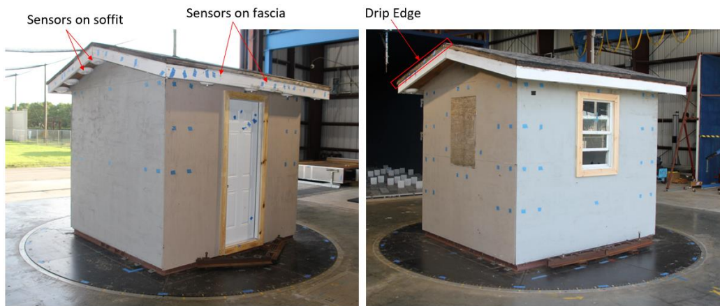
Figure 3. Scanivalve patches and wireless sensors attached to the soffit and fascia of the FIT house model.
